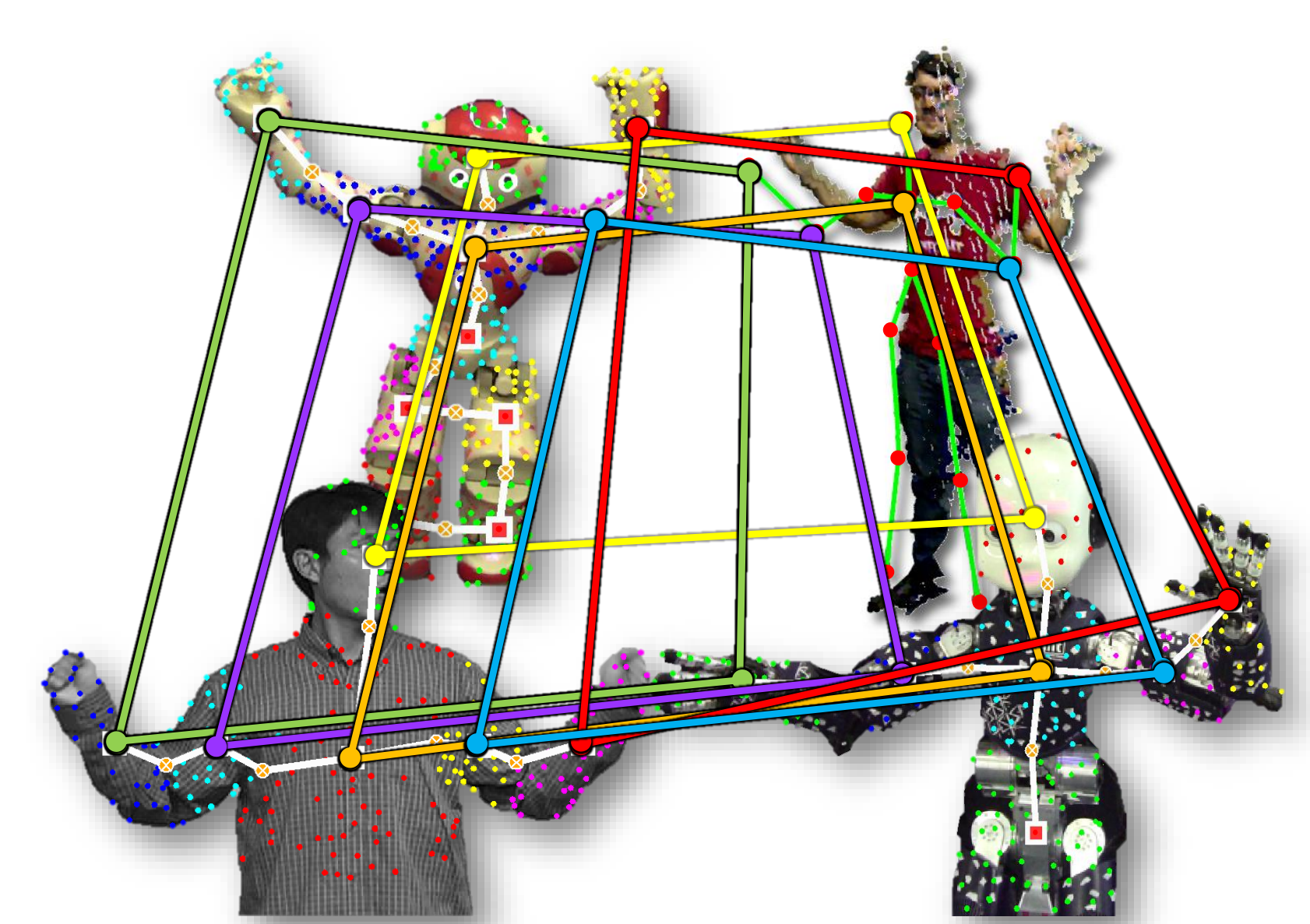
Figure 4: Kinematic Structure Corresp. Various kinematic structure correspondence matching results. The iCub humanoid robot (bottom right) can find correspondences to human partners, either sensed through the iCub eyes (bottom left) or a RGB-D camera (top right). Also, correspondences to other humanoid robots like the NAO robot (top left) can be found.
