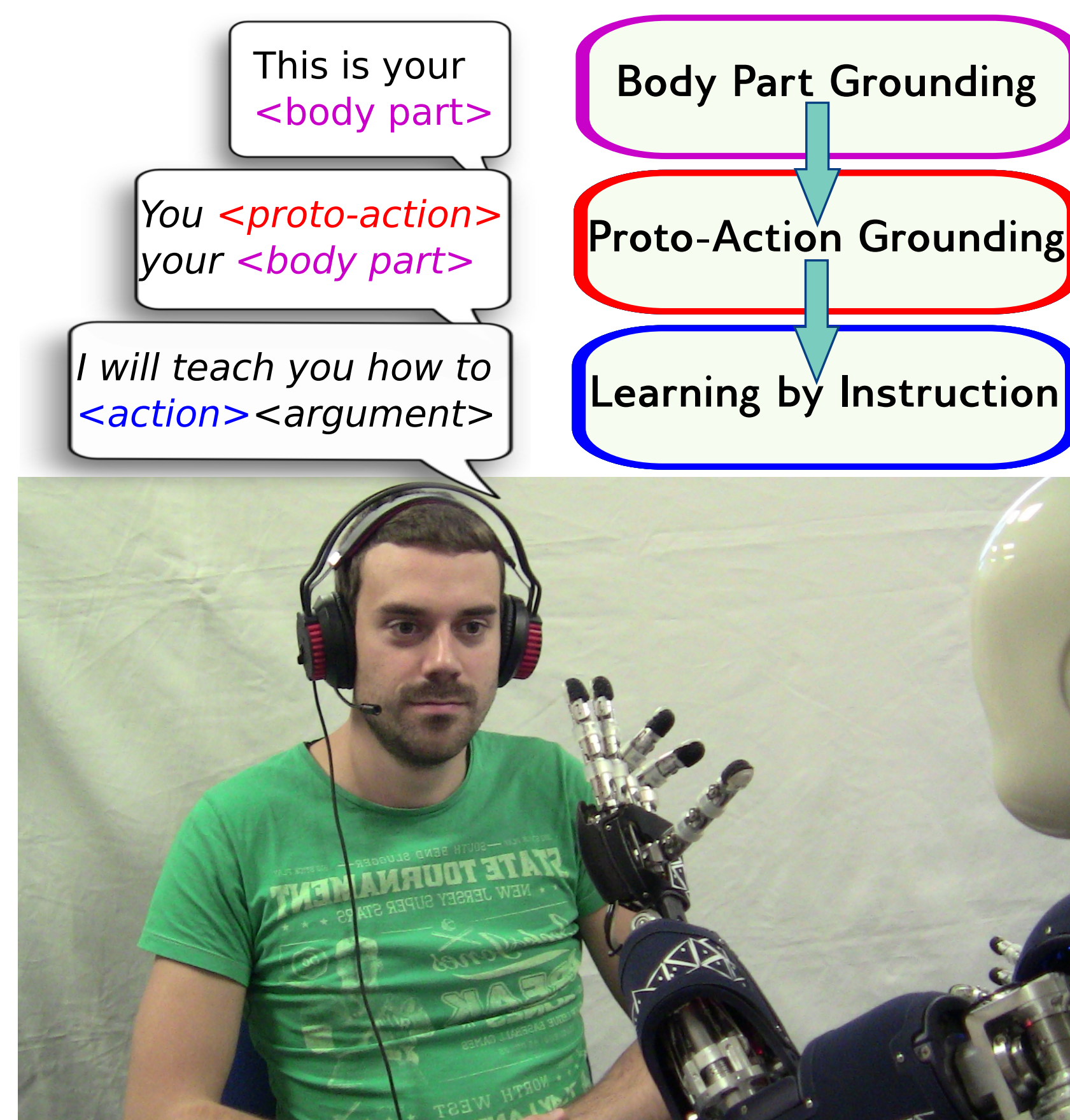
Figure 3: Symbolic Repr. Hierarchical components to 1) learn body part names from human labelling after a robot motor babbling, 2) discover proto-actions ( i.e. a single joint's position command) with on-the-fly descriptions by the human, and 3) learning by instructions with the human as teacher to scaffold the acquired skills into primitives or complex actions.
